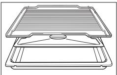
The anti-splash tray should be placed inside the deep sided grill pan when grilling or roasting.
